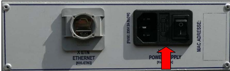
After switching off the device, always wait at least 5 seconds before switching it on again!
