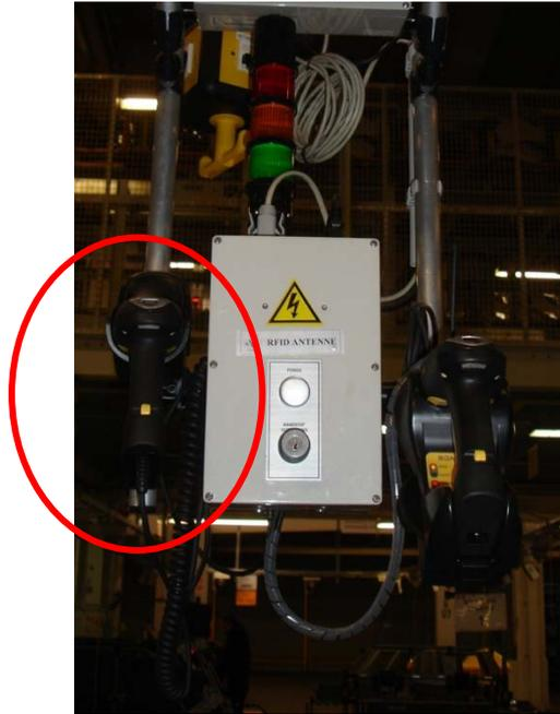
In case the cordless barcode reader is malfunctioning, use this device to scan barcodes from worksheets. (Nostrategy)
