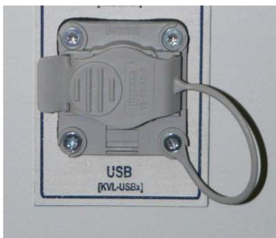
The USB connector built in on one side of the control box (VARIOSUB VS-A-F-IP67).
